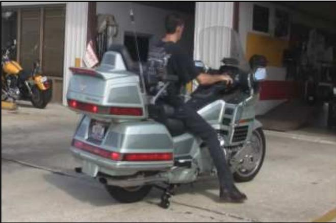
When using the LegUp® LandinGear System, the rider should stop the bike the same way they always did, and basically ignore the LandinGear!
