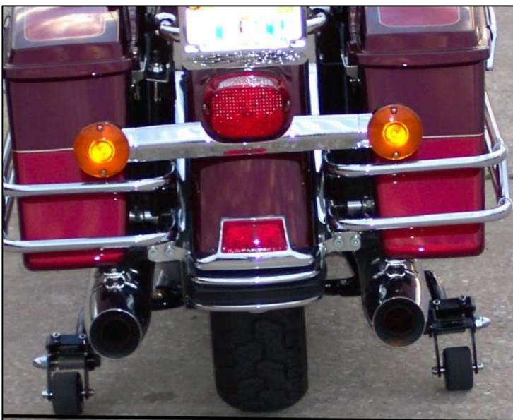
The system will **NOT** push the bike to the low side in this case, but will stop with the high-side wheel in touch with the ground, and the low side off the ground (picture at left). Your high side leg and the high-side wheel will combine for your stability and balance!
