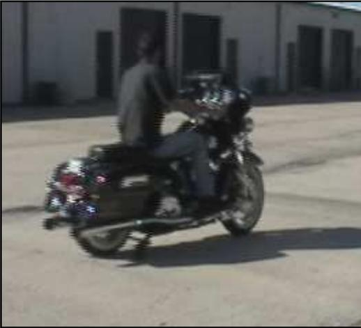
As previously discussed, the wheels of the system allow some leaning left and right when they are deployed. When it is time to leave, pull away from the light or stop sign as you normally would. The slower you leave, the longer the wheels will remain in contact with the ground, and vice versa. Using a normal speed will typically get the wheels up in a matter of a second or two!
