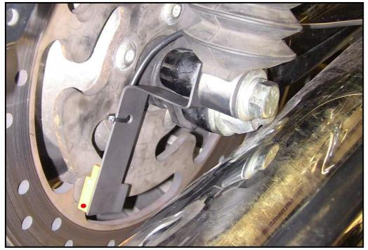
When you think you have it, turn the ignition to Accessory position, and roll the wheel to make the spokes of the rotor pass by the sensor. Each time one passes the sensor, the LED on the sensor should go bright then off.
