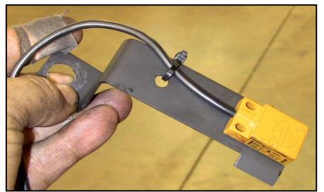
Remove the bottom bolt from the right shock at the rear of the bike. Insert the top of the bracket shown at left, behind the shock and in front of the hole in the swing-arm, so the bolt will pass though it when reinserted.
